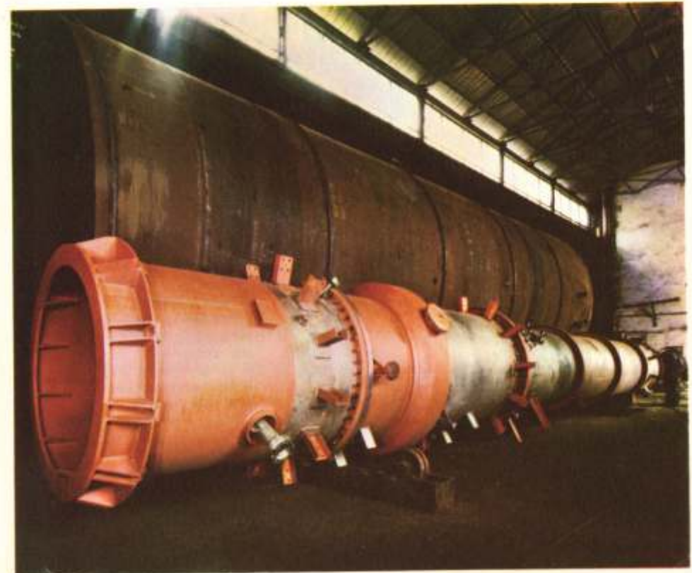
← 1.6 M dia X 16 M high stainless steel recovered solution rectification column under final assembly for Hindustan Fertilizer Corp. Ltd., Durgapur
